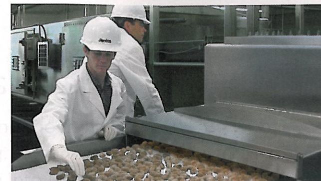
Meatballs and other protein foods benefit from microwave preheating prior to conventional cooking, increasing throughput and lowering operating costs for food manufacturers. Photo: Ferrite Microwave Technologies
